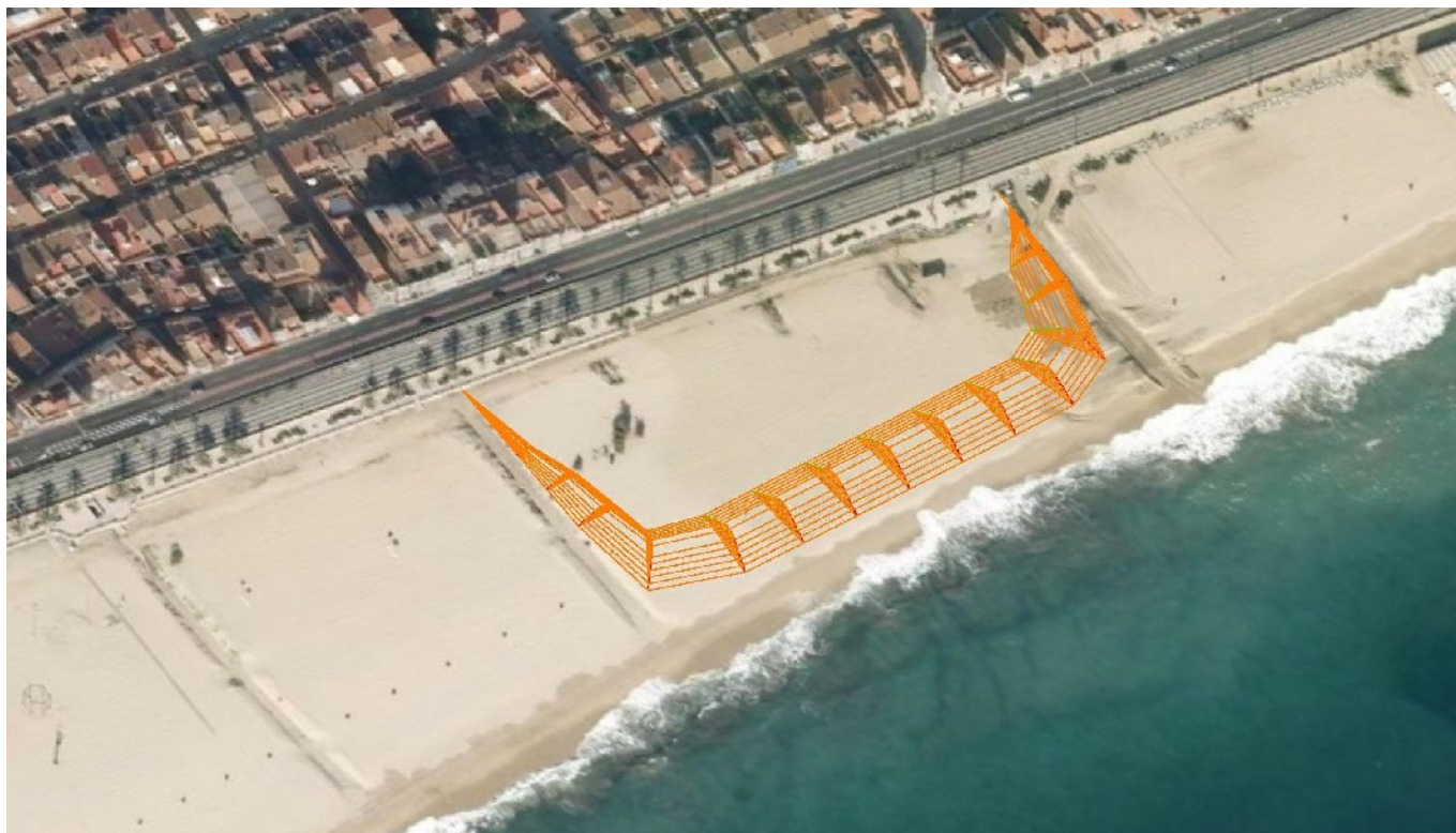
Aero-deflector sand dune project. Ocata beach.
